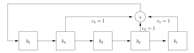
Example: Consider the following 5-bit linear shift register with the feedback equations
